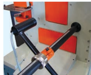
Electric back gauge
