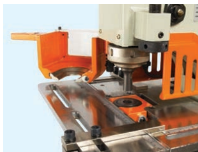
Swing away stripper for easy access and fast tooling changes.
