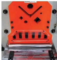
Shearing station with hydraulic hold down
