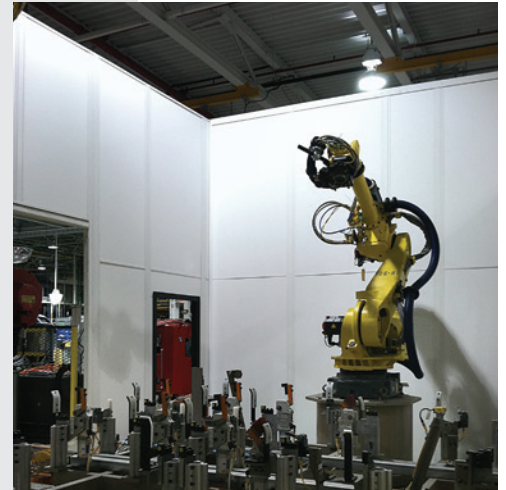
Protective Wall Partition System, 3" 16 gauge Steel Building System & 24 gauge painted Steel Wall Panels
