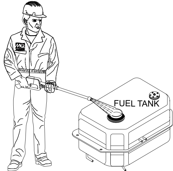
Figure 60. Fuel Tank Cleaning
