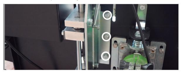
2. Also loosen the screws marked in the photos below and align the knife with the stop.
