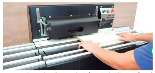
8. If necessary, you can increase the working area using the front extension table. Just pull or push, per your need.
