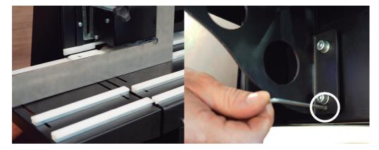
Adjustment is made by tightening or loosening the screw shown below. Remember that the adjustment must be made on both sides of the auxiliary table.
