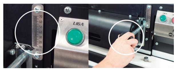
3. Also use the guides provided x 2 (one for each side) to make the height adjustment, according to the thickness of the MDF in which the treim will be made.
