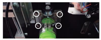
2. The height will be adjusted by turning the bolt shown below. Turning it clockwise, the router goes up, counterclockwise, the router goes down. After the height has been set, tighten the router's fixing screws again.
