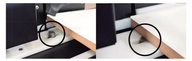
7. Guide panel along the equipment extension. Even though it has feed rollers, we recommend that you support the panel through complete trimming process by hand, especially with panels that exceed the size of the table.
