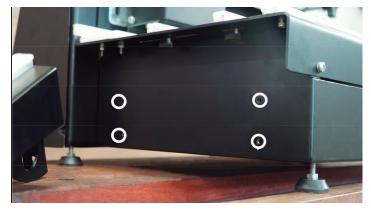
Each of the tables must be bolted on the threaded holes, indicated in the previous photo. Remember not to fully tighten before completely aligning the tables, following the next step.
