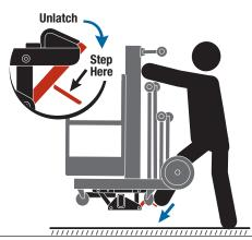
**3**. Continue to lower the PowerLift and Rocker Plate down until the Rocker Plate stops (**Figure 3-14**).
