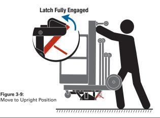
4. With the PowerLift resting fully on the Hitch Hauler Base Frame, insert Master Pin through both uprights and twist counter clockwise ¼ turn. Insert the Retaining Pin through the Rocker Plate, Master Pin, and Base Frame. Secure the Retaining Pin with either the Ring Snap Pin or Paddle Lock. Check that the pins are installed correctly by trying to twist the Master Pin. Master Pin should be locked from rotating (Figure 3-10).
