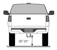
For vehicle receiver heights of 10"-15", place the Receiver Mount in the "Up" position into the vehicle receiver. For vehicle receiver heights of 16"-21", place the Receiver Mount in the "Down" position. Secure the Receiver Mount with the Receiver Hitch Pin, mounting as close to the bumper as possible (Figure 3-4).
