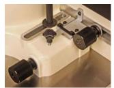
The fence system (left) is tough, stable and has all of the adjustments you need for safe, accurate shaper work. The right side fence face has this ultra-precise front-to-back control (right) for jointing-type operations.
