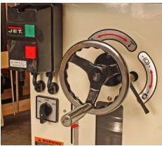
The powerful 3HP motor (left) and its mount are easily accessible through the side door. The major controls are on the front of the cabinet (right), including the magnetic switch that protect the motor and you.
