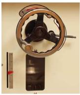
The handwheel and scale allow making precise cutter height changes quickly.
