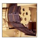
Caterpillar feed blocks constructed of special grade cast iron are heat-treated and travel on special hardened and ground "V" ways. Auto oiler with shut off insures long trouble-free convevor life. Variable feed speeds make it easy to get optimum feed/finish ratio.
