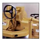
Job change over is fast and easy with convenient controls for height, width, conveyor and main blade. The 4" dust collection port is mounted right at the blade for improved chip collection and a clean work area.
