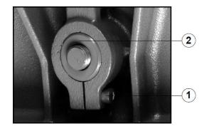
If there is insufficient blockage of the head arm in the desired position, loosen the screw (1) on the lever, hold the bushing (2) in position, turn lever left to tighten the screw.
