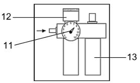
• Check the pressure by the pressure gauge (11) and use the regulator (12) to set the ideal pressure.
