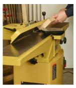
Whether used in the full vertical (left) or 45-degree position (right) in or out, the Powermatic 54A/54HH fence provides plenty of support for truly accurate cuts.
