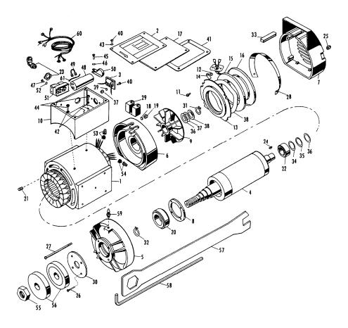
Each motor assembly includes items 1 through 61 depending on the phase of the motor.
