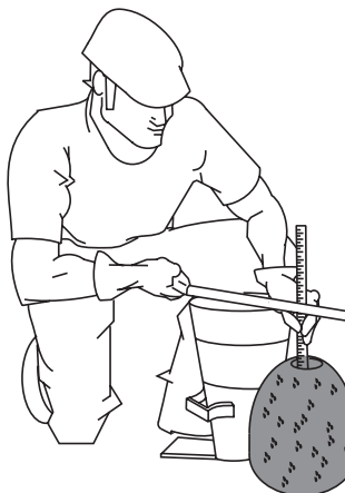
Figure 35-E. Slump Test (Cone Invert)
