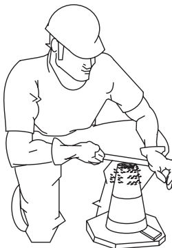
Figure 35-D. Slump Test (Removing Excess Concrete)
