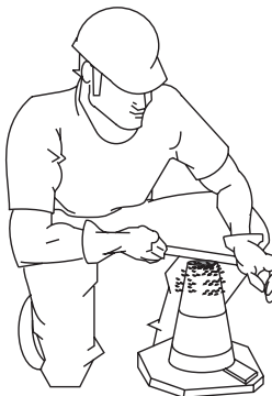
Figure 34-D. Slump Test (Removing Excess Concrete)
