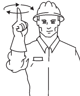
START PUMP SPEED UP
