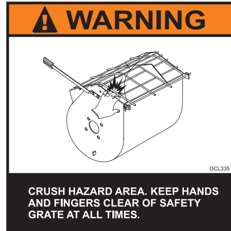
Figure 39. Safety Grate (Crush Hazard)
