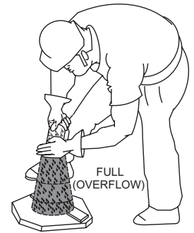
Figure 55-C. Slump Test (Full-Overflow)
