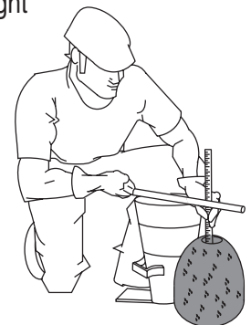
Figure 55-F. Slump Test (Measurement)
