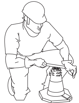
Figure 55-D. Slump Test (Removing Excess Concrete)
