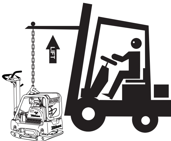
Figure 18. Lifting the Compactor
