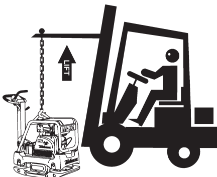
Figure 1. Lifting the Compactor
