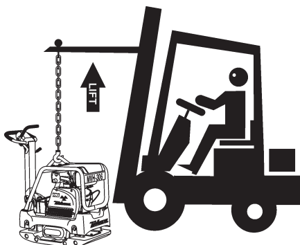
Figure 18. Lifting the Compactor
