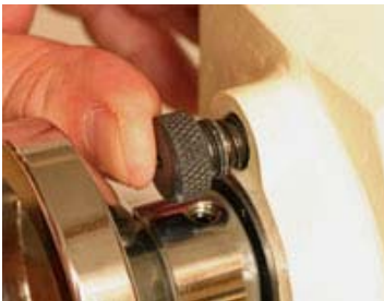
This simple button can be pushed for temporary spindle locking or screwed into any of 24 positions for various routing or drilling operations.
