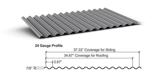
Corrugated Panels come in different rib heights, but the most popular is 7/8 Corrugated. This profile has 2.67" on center and is 7/8" tall on the ribs.
