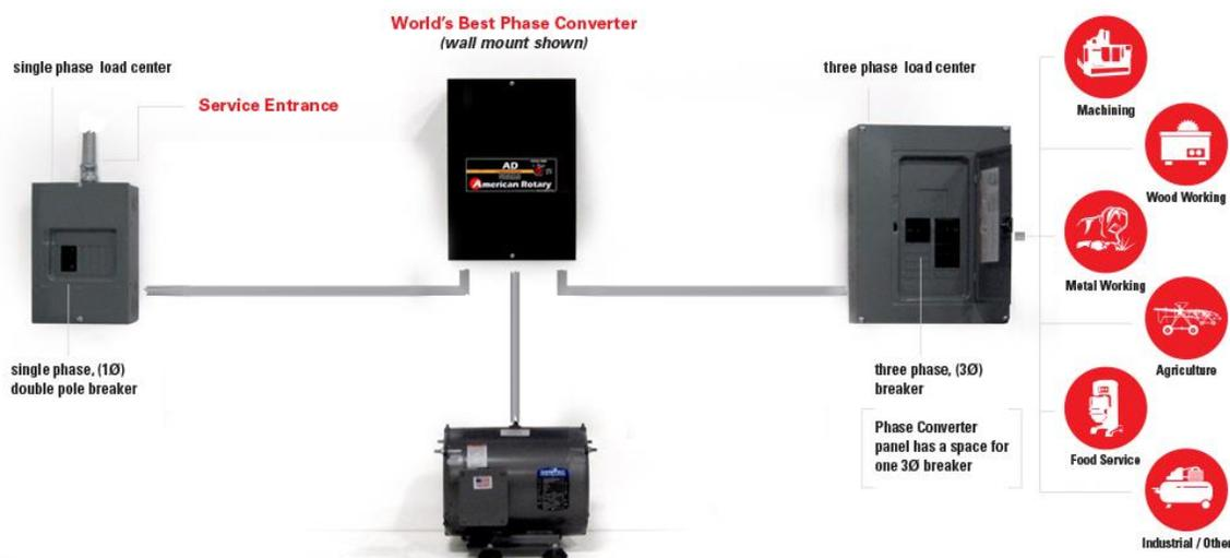
An additional 3-phase breaker panel may be installed on the line between the converter control panel and the 3-phase equipment. This is recommended to protect each piece of equipment and the wire that feeds that equipment.
