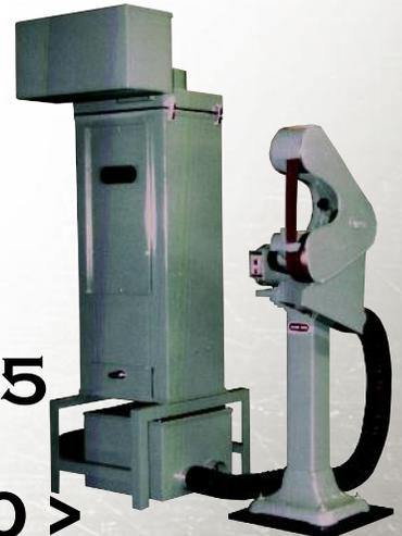
Burr King dust collectors use space saving cabinet design. All Burr King grinders/buffers may be coupled to these efficient dust collection systems. Select the BK 75 or BK 125 for portability or the BK100 for two grinder/buffer, fixed installation. Includes silencer and spark boxes. Machine sold separately.
