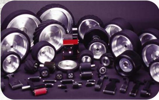
Grinders/buffers capability is readily expanded by selection of the best contact wheel/buffing wheel combination for your material. Many contact wheel diameters, widths, hardnesses and face geometrys are available - 55 shore, for general purpose grinding, 90 shore serrated for heavy grinding. Numerous nylon wheels, buffing wheels and specialty wheels are available. Consult with the factory for proper selection.
