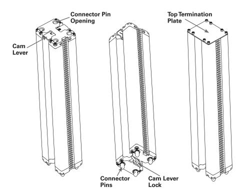
Figure 2.8 - Mast Connectors
