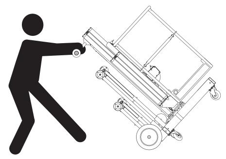
Figure 3-8 Maneuvering when tilted back
