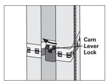
**2.** Rotate the cam lever lock until it stops in the center position.
