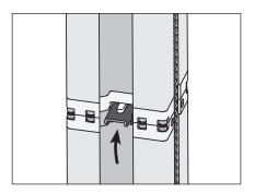
**3.** Release the cam levers to the open position.
