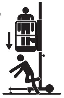
Warn personnel not to work, stand or walk under an elevated platform. Position barricades on the floor as necessary.
