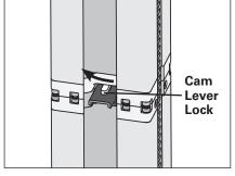
**2.** Rotate the cam lever lock until it stops in the center position.
