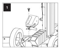
Remove retraction winch from chassis.
