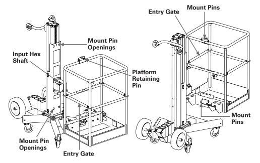
Figure 2-7 - Platform Mounting and Retaining Pins
