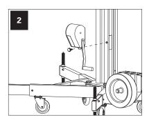
Attach winch to base mast and unwind strap.
