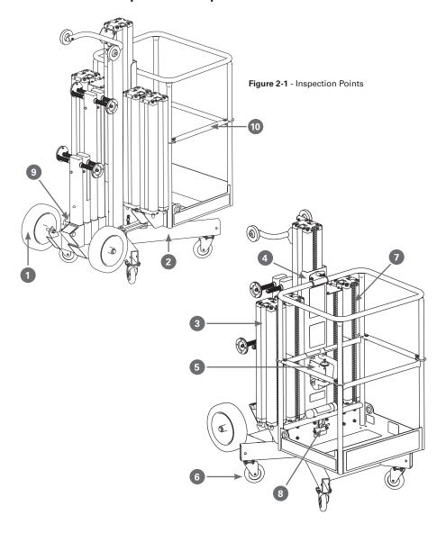
NOTE: On all components, make sure there are no loose or missing parts and that everything is securely fastened. Make sure that there is no visible damage or excessive wear
