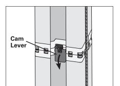
1. Press both cam levers inward to allow the cam lever lock to rotate freely.
