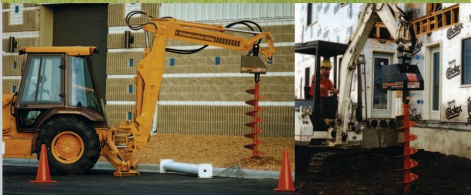
General's 671 DIG-R-TACH... derives power from the auxiliary hydraulic system of the carrier vehicle.
