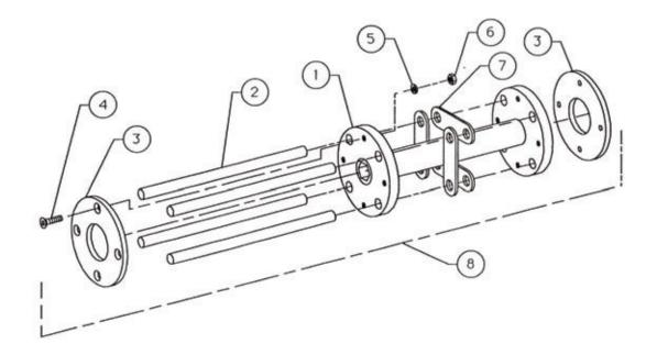
**Two Section Drum Assembly SP8 Series II Surface Planers**
