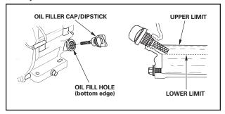
The necessity of using the correct oil, and keeping the crankcase full cannot be overemphasized. Engine failures resulting from inadequate or improper lubricant are considered abuse and not covered by the generator or engine manufacturer's warranty.
