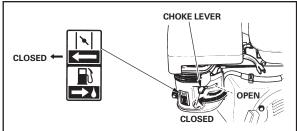
Move the choke lever to the "CLOSED" position.
