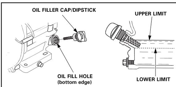
Oil is added to the engine through this oil fill hole. After filling the crankcase to the proper level, be sure you properly tighten the oil filler cap/dipstick.
