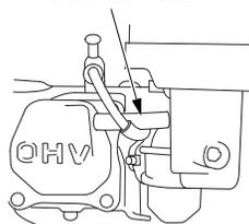
1. **Change the oil** after the first 20 hours of operation and yearly or 100 hours thereafter under normal operating conditions. Change engine oil every 50 hours of operation if the engine is operated under heavy load, or in high ambient temperatures.
