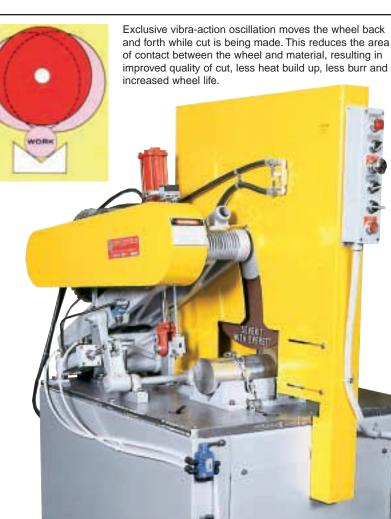
Dry Cutting Speeds (average) Size Material Time 6" Solid 115 sec. 8" x 8" Anale 20 sec. 12" Channel 40 sec.
