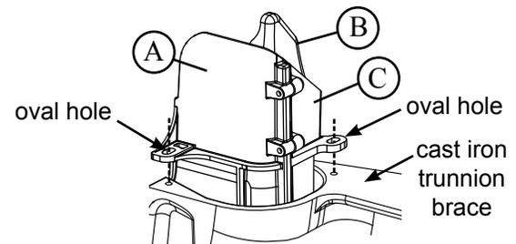
**10.** Turn the elevation handwheel to lower the arbor all the way down.
