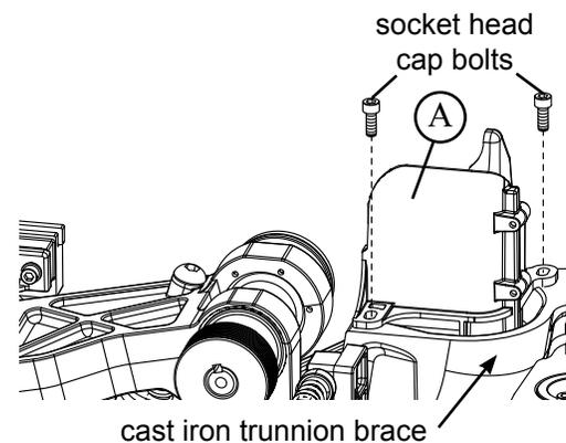
**12.** Turn the elevation handwheel to fully raise the arbor and re-install the blade. The arbor must be raised when installing a blade with the new dust shroud installed. Close the dust shroud door and re-install the table insert and blade guard.
