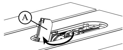
Now maneuver the upper portion of the left dust shroud half around and to the front of the arbor and move it to the left side of the cast iron trunnion brace, but do not fully seat it in the saw. Rather, raise the upper portion so that the screw bosses are above the table surface to more easily install the blast shield.
