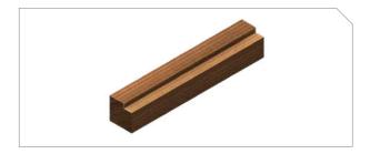
A rabbet cut is used to create a rectangular notch along the edge of a workpiece.
