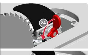
Rotate clamp handle down (2A, 2B) to secure riving knife in place. Install table insert. Reverse steps to remove riving knife.
