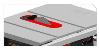
Stop motor and turn saw off. Remove wood and clamps. Remove table insert and install riving knife or blade guard (see page 30). Reinstall insert.
