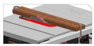
Start motor and slowly raise blade to highest elevation. This will widen slot for beveled cuts up to 45 degrees.
