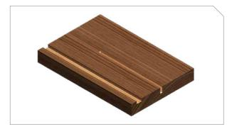
Groove cuts are like Dado cuts and used to create a slot or trench in the surface of the workpiece. However, unlike Dado cuts, a groove is cut parallel to the grain of the workpiece.
