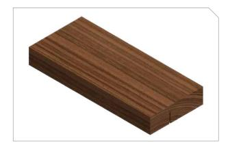
A non-through cut does not extend through the entire thickness of the workpiece. In this case you cannot use the blade guard and splitter but must use the riving knife instead.
