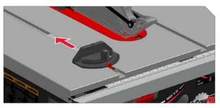
Slide the miter gauge into either miter slot in table top.
