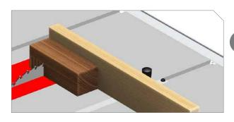
Make a series of evenly spaced cuts along workpiece, moving workpiece over slightly between each cut.
