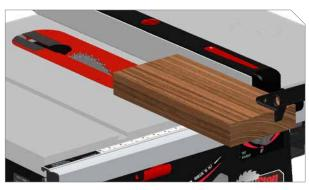
Remove the blade guard and install the riving knife (see page 33). If the non-through cut is a rip cut use the fence.
