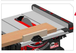
To reduce the potential for kickback and serious injury, move the fence out of contact with the workpiece when cross-cutting to prevent the workpiece from binding between the fence and the blade.
