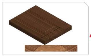
A plunge cut is used to create a slot or opening somewhere other than the edge of the workpiece.
