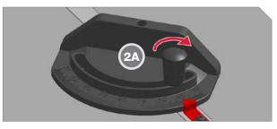
To adjust miter gauge angle, turn lock knob counter-clockwise, and then pivot miter gauge head until red pointer is above desired angle (+/- 60°). Tighten lock knob by turning it clockwise (2A) before making cut.
