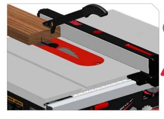
Use the riving knife for every operation where the blade guard cannot be used. Neither the blade guard nor riving knife can be used when making Dado cuts.
