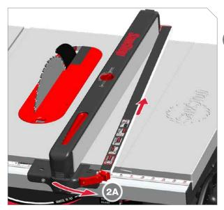
Store low fence on right side of rip fence. Low fence can be used on either side of rip fence. To use low fence on left side of rip fence, pull lever forward (2A) and slide low fence slightly back to unhook rear.
