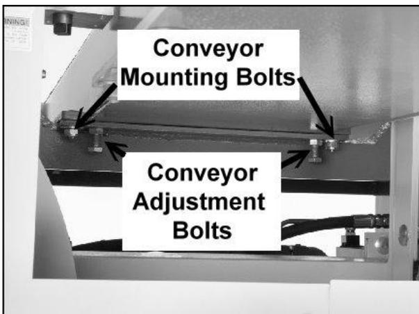
4. To raise the left side, loosen the lock nuts on the conveyor adjustment bolts on the left side and tighten the adjustment bolts. Do the same procedure to the right side bolts to raise the right side.
