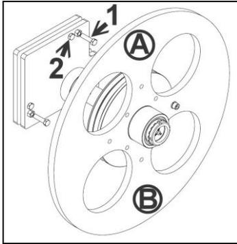
There are two adjusting screws. To adjust the screws will make the saw wheel surface slide. The purpose is to fix the position of (A) and (B).
