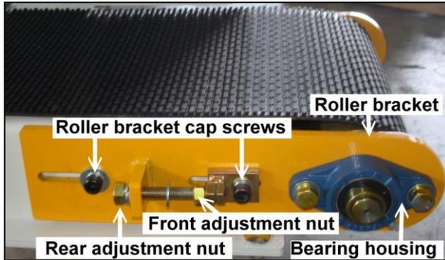
1. Loosen the two roller bracket cap screws on the both side of the conveyor about 3/4 of a turn.
