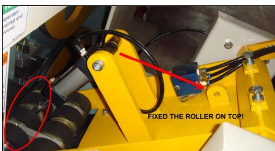
**Make sure to lift up the front roller and fix on top when saw blade is higher than 60mm, nor the roller will be cut by blade!**
