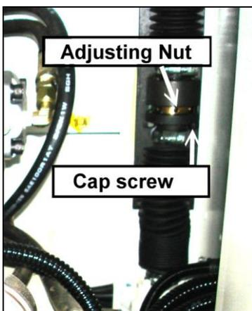
8. The adjusting nut shown in raises, or lowers, the non-drive side of the bandsaw blade (the side opposite the motor). Insert the pry tool into the adjusting nut.
