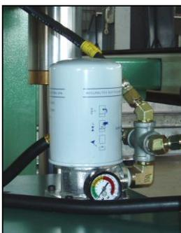
6. Separate the filter from the filter housing by pulling them apart.
