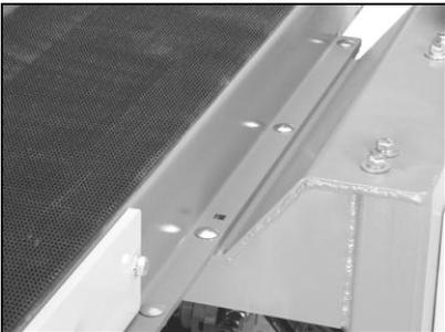
5. Look under the conveyor for the carriage bolts. Place the flat washers and lock nuts on the carriage bolts and tighten.
