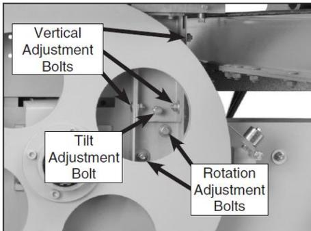
3. Shift the blade guide adjusting bracket until the blade is centered in the guide slot.
