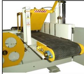
3. Lift the conveyor belt onto the resaw body as shown in the right.
