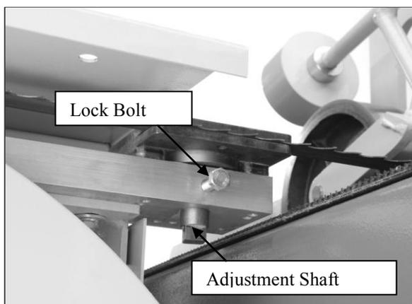
2. Rotate the adjustment shaft until the support wheel is approximately 0.016" behind the back of the blade. Check with a feeler gauge or four thicknesses of a dollar bill.
