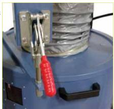
Quick release lever lifts the lid from the drum allowing it to be quickly rolled out and dumped.
