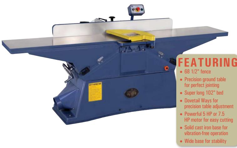
The Oliver 4270 16" Jointer is ready for anything you can throw at it. With 16" of jointing capacity you'll be hard pressed to find a job that outclasses this beast. With a super long 102" bed and an ample 68 1/2" fence, your stock comes out straight and true every time. A powerful 7.5 or 5 horsepower motor gives you the torque you need to joint the toughest hardwoods with ease.
