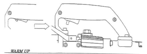
In cold weather, warm up unit for 30~60 seconds so that the hydraulic oil reaches the proper viscosity. Pull trigger switch to extend piston and release when it has reached its full stroke. Repeat 3~5 times.
