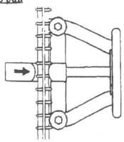
Set the hook in the correct starting position, make sure that the mode control lever is in the "B" position and fit the rebar as illustrated. Pull the trigger switch until the desired angle is attained.
