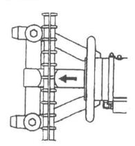
Advance or retract the piston so that the hook is in a suitable starting position. Set the mode control lever to "A" and fit the rebar as shown at left. Pull the trigger switch until the rebar is at the desired angle.
