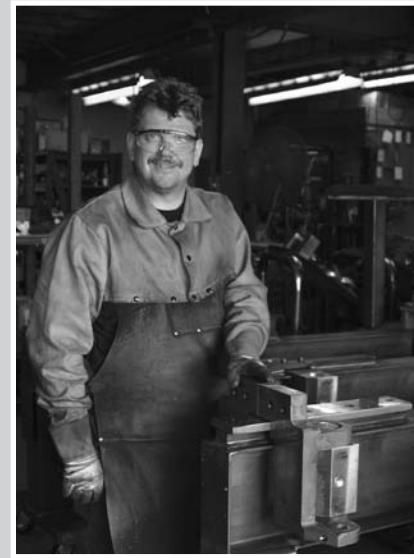
Mark Jeffords with the welded heavy-duty I-beam frame for a Huth bender.
