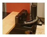
The full-featured miter gauge fits the slots in either table.
