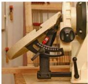
The cast iron table mounts on a single rod that can also be installed at the belt section. The table tilts to 45-degrees and features a handy
