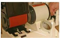
In addition to the 4"-diamter dust port, we included dust gates at the disc and belt section to maximize the suction where you need it.
