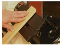
With the belt in the upright mode, the table can be tilted up to 45-degrees for precise trimming or forming. The miter gauge fits both the cast iron disc and this aluminum belt table.
