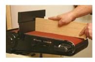
The belt can be positioned flat, as it is here or fully vertical.
