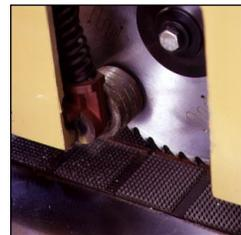
*The 12" blade is supported by a Ni-Cr-Mo alloy heat-treated arbor that is precision ground and dynamically balanced. Four large diameter bearings support the arbor and a full 15 HP is delivered to the cut. Five spring-loaded hold-downs insure accuracy.*
