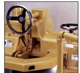
*Job change over is fast and easy with convenient controls for height, width, conveyor and main blade. The 4" dust collection port is mounted right at the blade for improved chip collection and a clean work area.*
