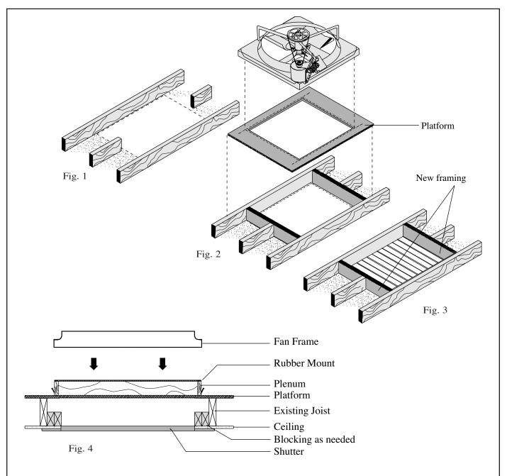
"CSS" SERIES SHUTTER INSTALLATION Models CSS-24, CSS-30 & CSS-36, install on joists with 16" or 24" centers.
