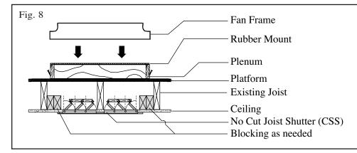
**STEP 10.** Install the flush mounted ceiling shutter into the ceiling opening using the screws provided. Caution should be taken not to effect the free operating action of the shutter. (See fig. 8).
