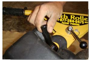
hose ends you previously installed and switch ends on the hoses. This is due to flow control purposes: although most sources are designed to flow in both directions, the curb roller contains a directional check valve installed inline for flow control purposes. After you have completed switching the hose ends, plug the curb roller back into the source and try again (starting with Step 6).
