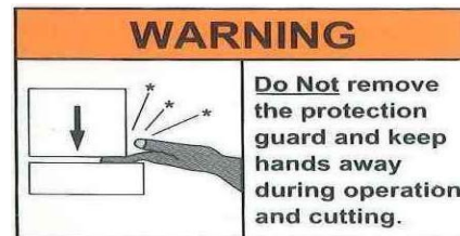
Figure 10. Guarding label – do not remove guarding & keep hands away from point of operation
