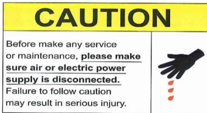
Figure 3. Disconnect Power label
