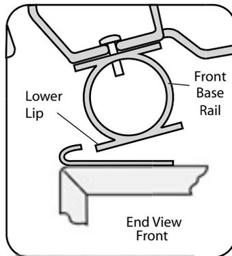
Place the lower lip of the front brake base rail into the opening of each retainer. With lip securely in place, lower brake onto mounting surface.
