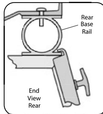
Extend each latch plate up and over the lower lip of the rear base rail as shown above. Tighten "T" knobs firmly to secure brake to stand.
