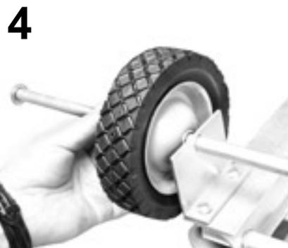
Insert axle through flat side of wheel hub. Next, insert axle through both bracket holes.
