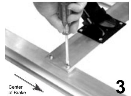
After ensuring the channel of the leg strut is facing downward, align the holes in the mounting plate with those in the base rails. Insert the remaining slotted hex screws through holes until snug. Repeat step with opposite leg assembly. Legs should now extend straight up from rails (after locking struts).
