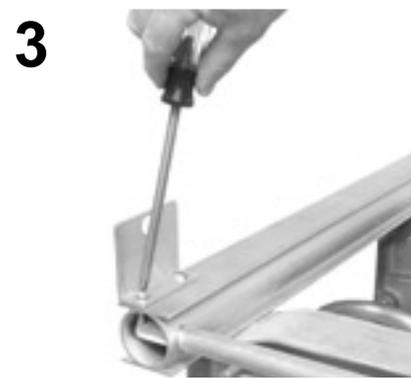
Install screws through both brackets and into each corresponding base rail using a Phillips type screwdriver.
