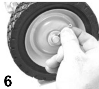
Insert washer onto axle until hole is clearly visible. Insert cotter pin through hole and spread apart.
