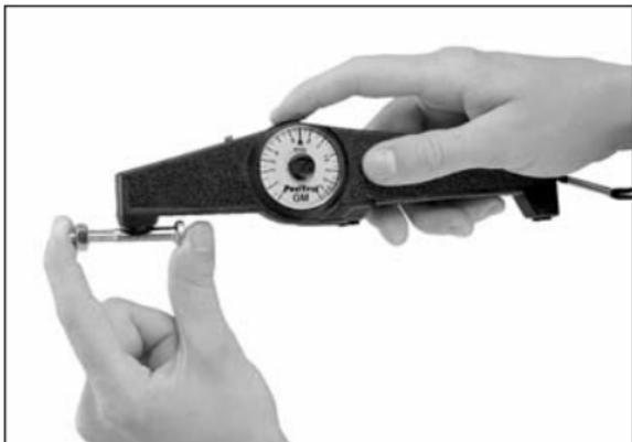
**Note:** *PosiTest* is available in two measuring ranges and in mils or microns scale.
