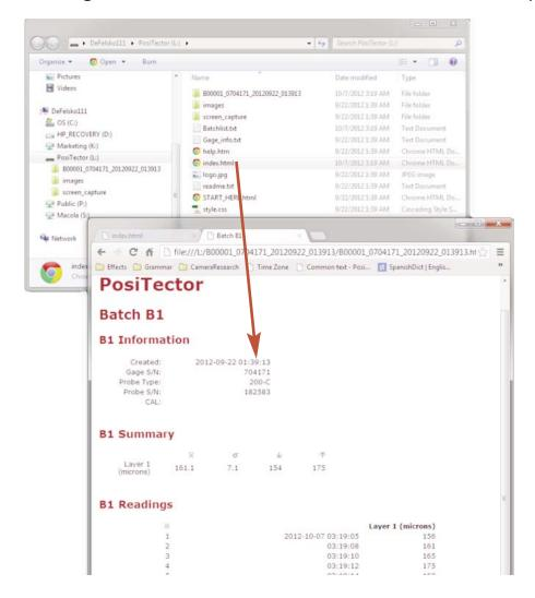
When your **PosiTector** is first connected to your Windows PC via a USB cable, an enumeration process is started that installs device drivers without re-booting your computer. You may see several pop-up windows in the taskbar at the bottom right of your screen. Wait for the entire process to be completed before proceeding.
