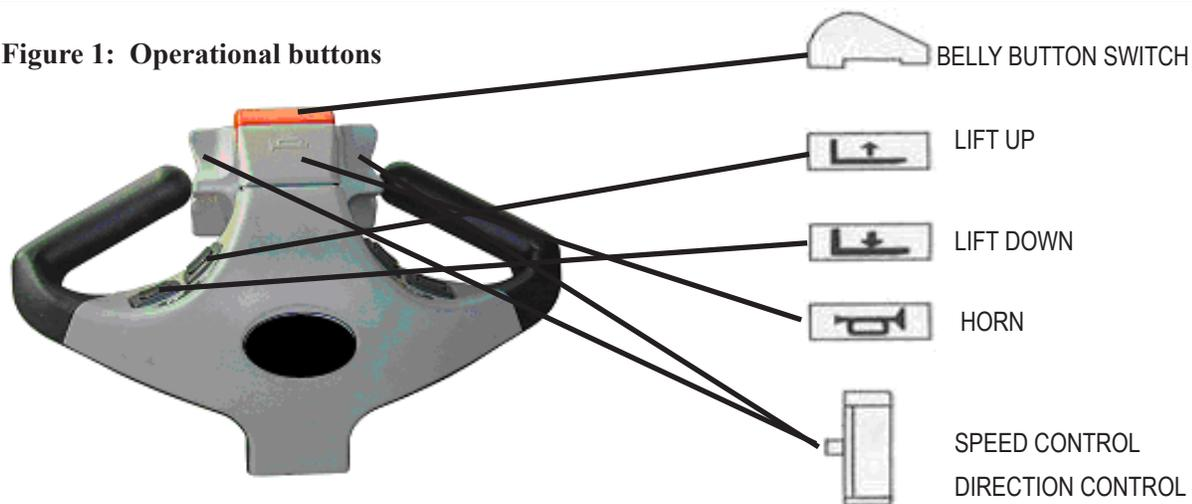
path of travel is clear of people. Never carry loads above the loading capacity of the stacker. It is suggested that when traveling without a load, the forks be in the lowered position. The speed of the stacker is increased by the degree of the rotation in either direction; it functions like a throttle. When you release your hand from the butterfly control, it automatically will resume to the neutral position and the speed of the stacker will slow down.
