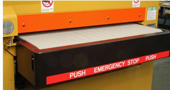
A disk brake stops the machine quickly when the OFF button is pushed or the emergency Stop bar is bumped.
