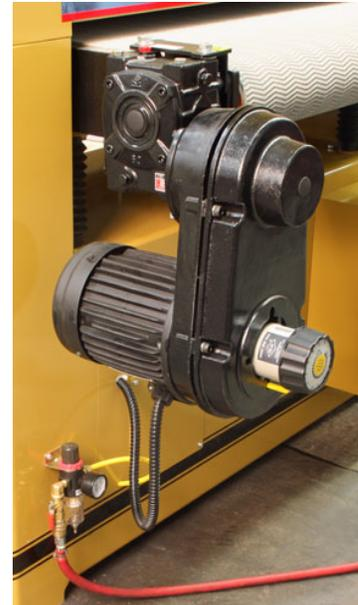
The feed conveyor has its own variable speed motor and an infinite control.
