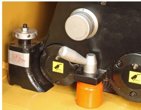
Belt changing is fast and tool free. A dial control shuts off air pressure to the tensioning cylinders to free the belt, remove the spacer block and the belt slips off of its rollers. Slide the new belt into position, install the spacer block and apply air pressure to tension it for use.
