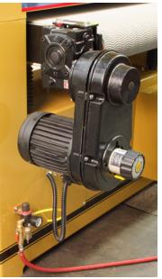
The feed conveyor has its own variable speed motor and an infinite control.
