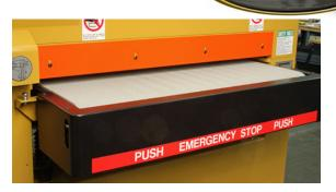
A disk brake stops the machine quickly when the OFF button is pushed or the emergency Stop bar is bumped.
