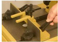
Even the fence is locked in position with finger-operated levers.
