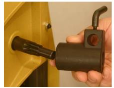
Moving the operating arm from the right To left sides is simple and tool free.
