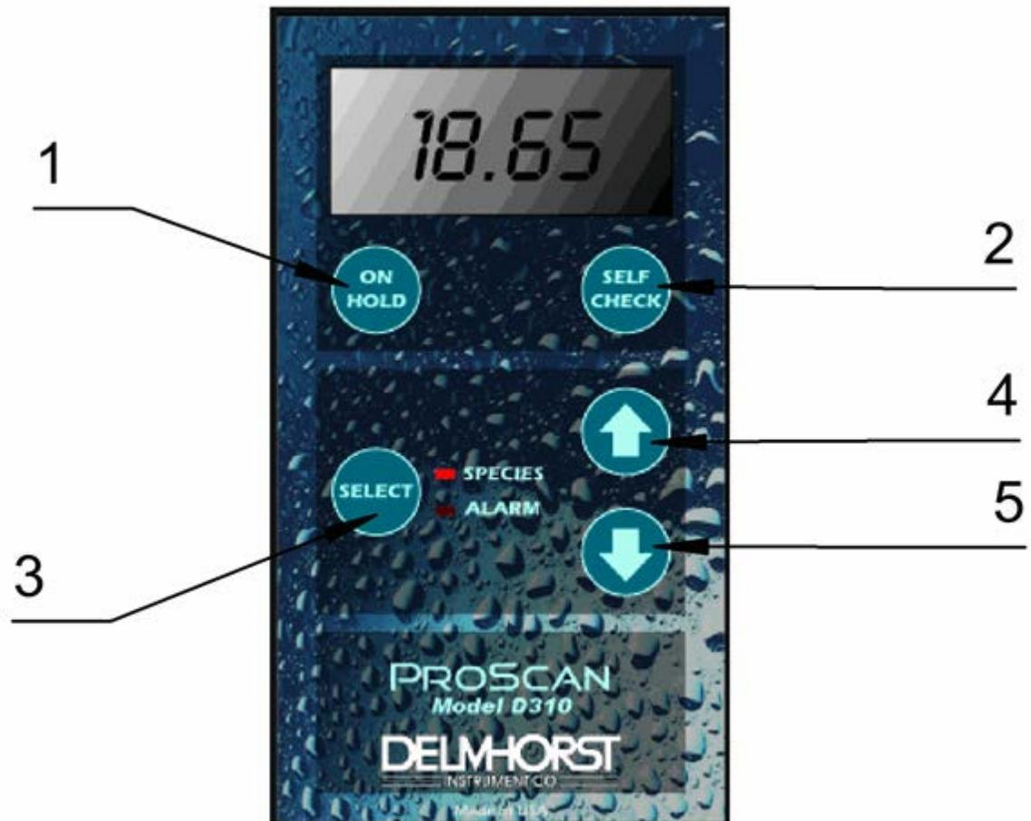
1. **On/Hold Key:** Press to turn meter on, return to reading mode after checking calibration, setting alarm, or to hold the current reading if pressed while reading. (There is a slow beeping sound while holding a reading.)
