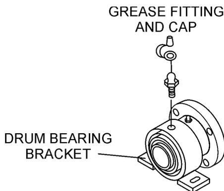
Figure 24. Grease Fittings (Dumping Mechanism)
