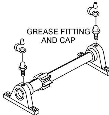
Figure 25. Grease Fittings (Countershaft)
