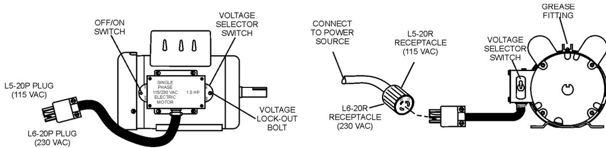
**Figure 4. Single-Phase Electric Motor
