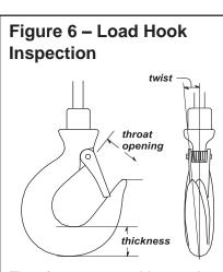
The wire rope assembly must be replaced if the throat opening is 15% wider than nominal, if the thickness is 10% less than nominal, or if the hook is twisted 10° or more. f
