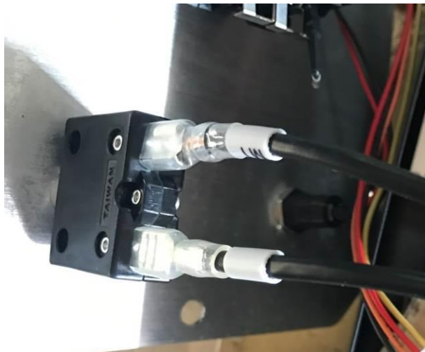
Figure 13: Removing 110V Overload Protector
